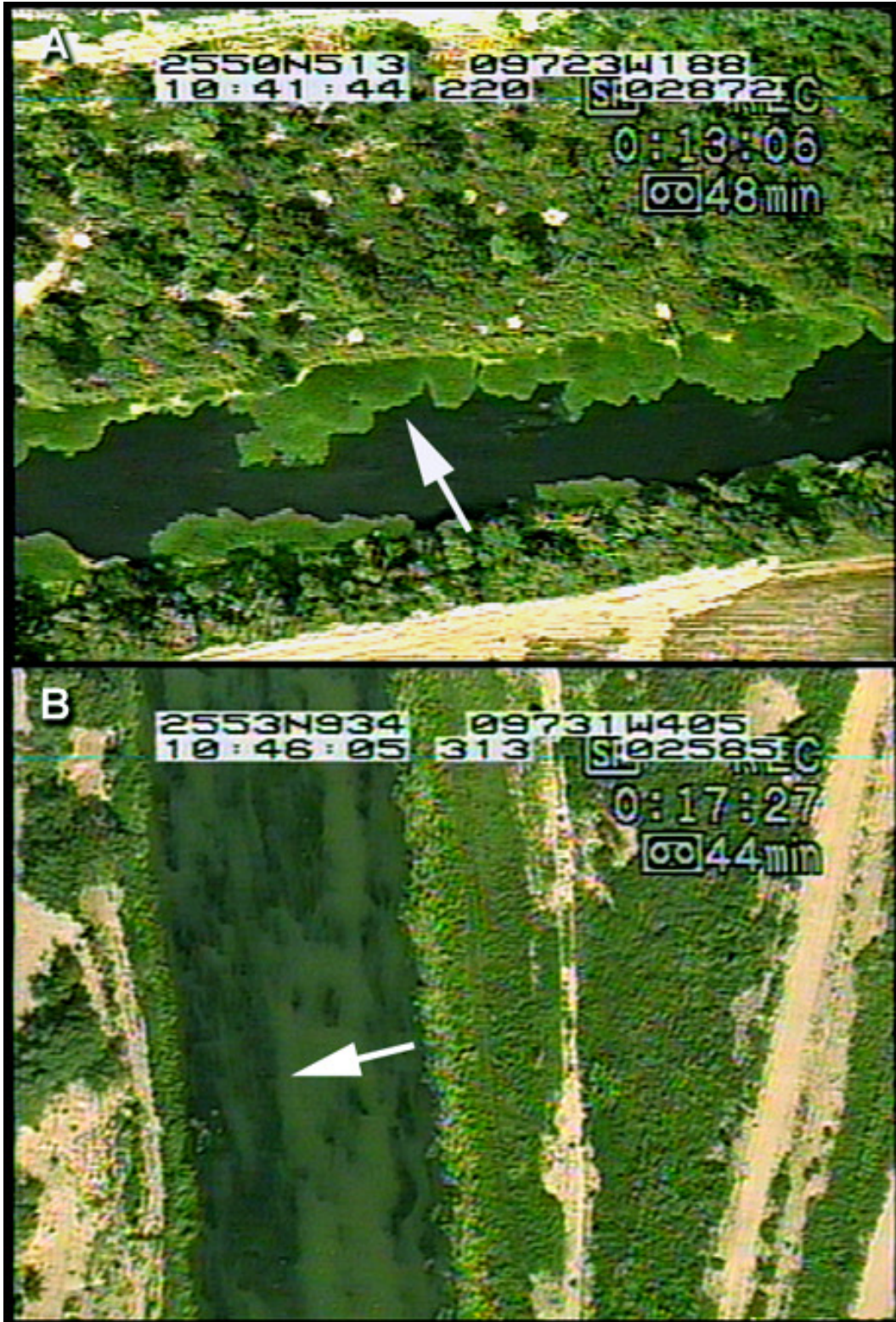
Fig. 1. Aerial normal color video images of infestations of waterhyacinth (A) and hydrilla (B) in the Rio Grande near Brownsville, Texas. The arrows point to waterhyacinth and hydrilla in each respective image. The imagery was obtained on September 19, 2002 at an altitude above ground level of approximately 600 m and had an original pixel size of approximately 0.70-m.
