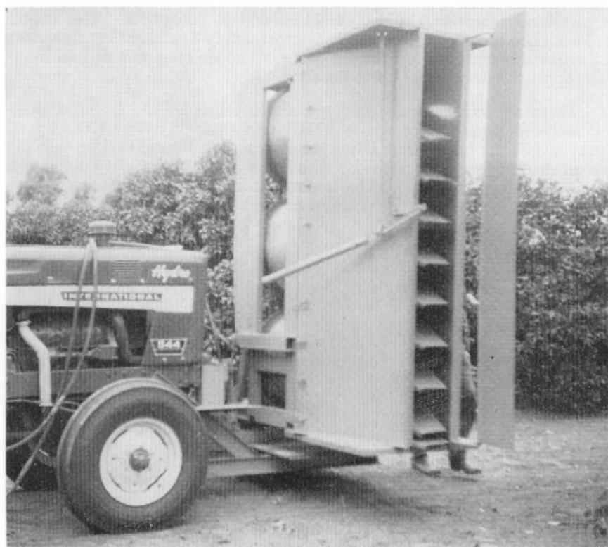
Fig. 3. Experimental air blast tree shaker with manually operated vertical and louvers in air discharge outlet.
