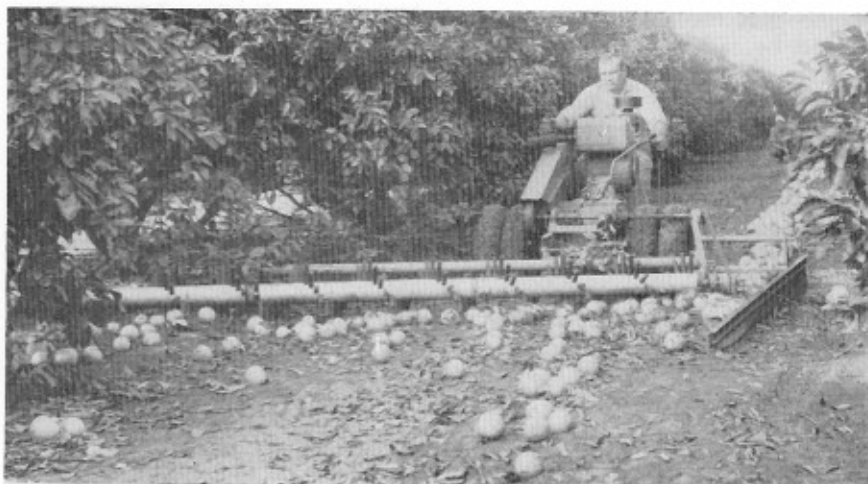
Fig. 1. Experimental citrus sweeper, used for sweeping both the debris for pick-up for disposal and for windrowing harvested fruit for loading into an orchard transport.
