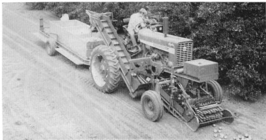
Fig. 4. Experimental citrus loader for loading windrowed fruit into orchard transport.
