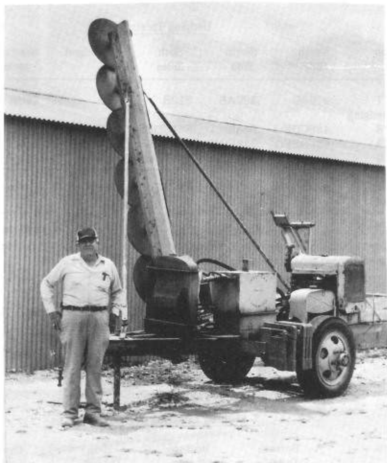
Fig. 1. Hedging machine constructed at Texas A&I Citrus Center. The 14 ft boom holds seven 28-inch diameter circular blades powered by a 46 HP engine.
