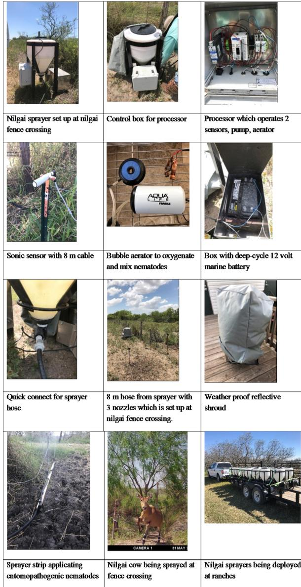
**Figure 1.** Remotely operated nilgai sprayer
