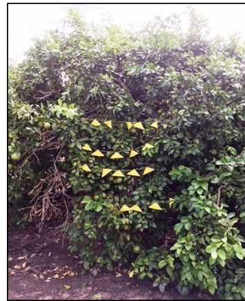
Fig. 3. Plasticized PVC infused with beta-cyfluthrin exposed to weathering by deployment in a citrus tree canopy.
