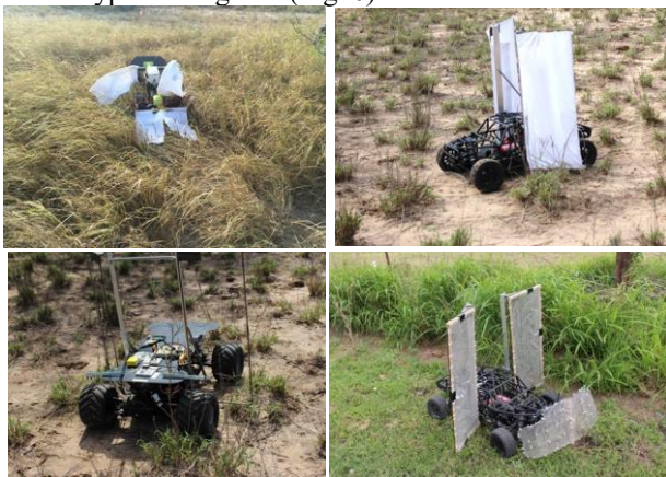
Figs. 3-6: 3. Tick-bot version 1.0, the Virginia creeper. 4. Tick-bot version 2.0, the Texas rover. 5. Tick-bot version 3.0, high-tech rover provided by VMI. 6. Tick-bot version 4.0, cluster-buster.
