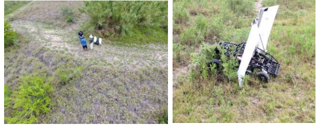
Figs. 10-11. Drones eye view of the tick-bot and the operator. Tick-Bot 2.0 high centered on Borrichia at Laguna Atascosa.
