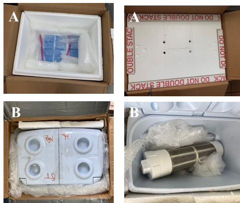
Fig. 3. (A) The cardboard shipping container measures (0.762m x 0.558m x 0.432m) [30in x 22in x 17in] with an inner styrofoam box and multiple icepacks. (B) The secondary shipping container (0.635m x 0.457m x 0.457m) [25in x 18in x 18in] for one PVC canister stored in an Igloo TM hard-sided ice chest.
