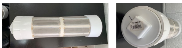
Fig. 4. The fruit were packaged in specially designed PVC canisters to contain any escaped larvae from the fruit during transportation.
